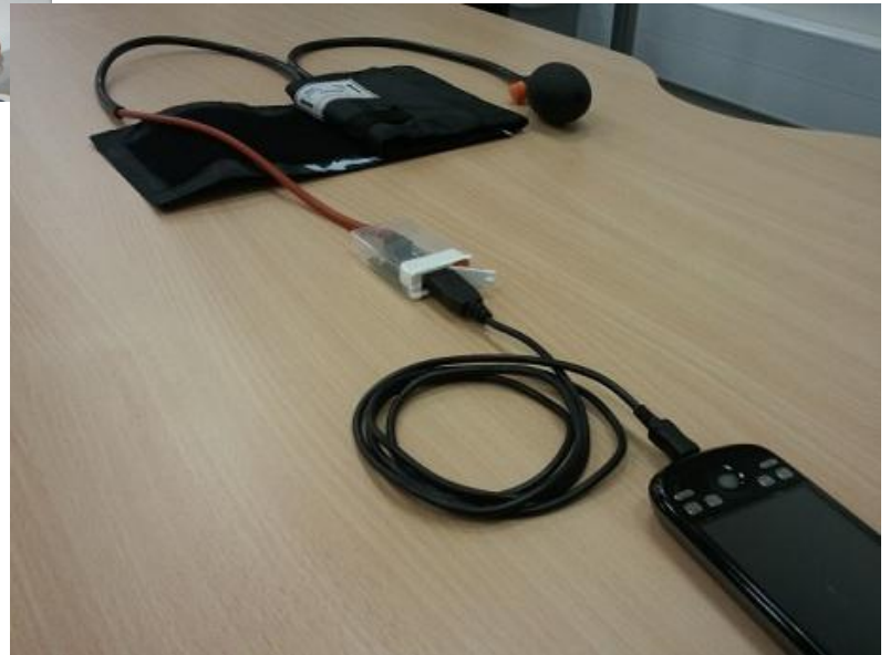
The winning Design Competition entry. A blood pressure monitor powered by a cell phone! Submitted by the BP team from Oxford University in the UK.
