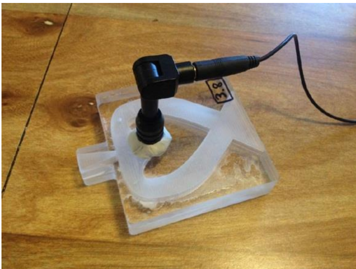
The 2012 EWH Design Competition winning device was a low-cost spirometer, a tool used in diagnosing and monitoring respiratory diseases.
