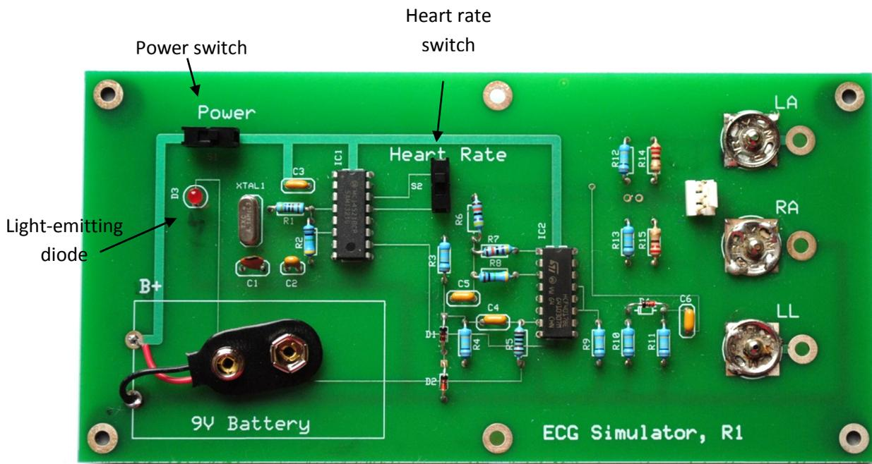
Figure 21 – ECG Simulator Kit after assembly.
