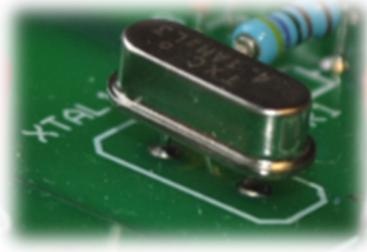
Figure 16 – Placement of the 4.1943 MHz crystal in the printed circuit board.
