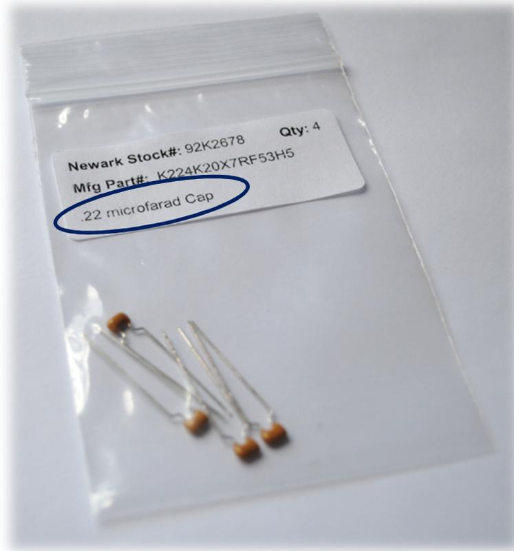
Figure 5 – Component description in value in the bag label.
