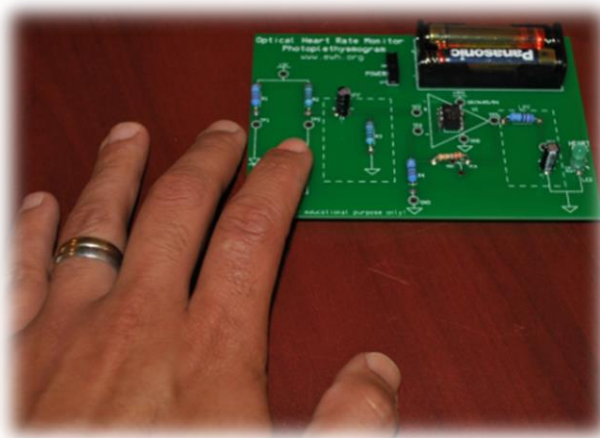
Figure 25 – Heart Rate Monitor fingertip measurement, the circuit works better if your elbow and all fingers lay on the table.
