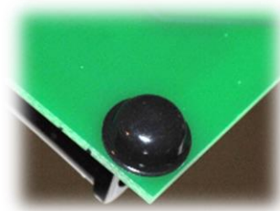
Figure 22 - Rubber feet to be placed underneath the corner holes.
