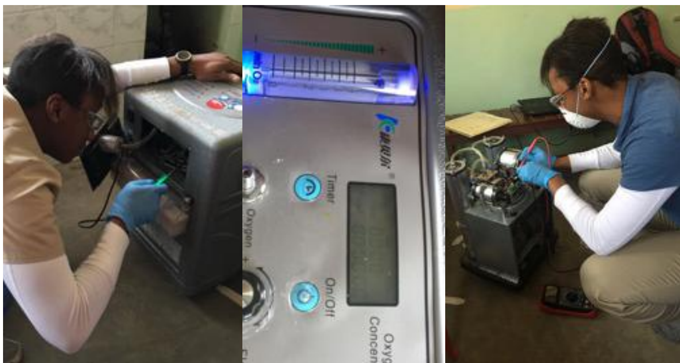
Left: Leah Putman troubleshooting an oxygen concentrator, Middle: Error on Oxygen Concentrator being worked on photo on the left, Right: Leah Putman troubleshooting another oxygen concentrator
