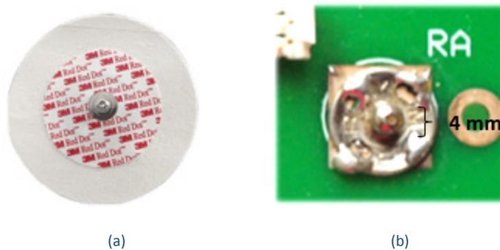
Figure 19 - Disposable patient ECG electrode 4 mm contact (a) and sew-on snap soldered to the Kit board (b).
