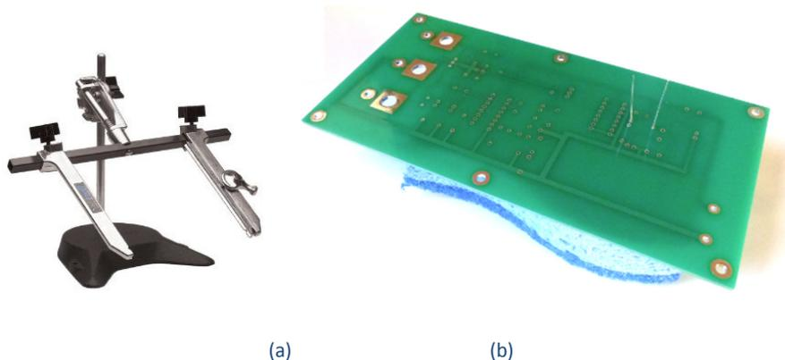
Figure 8 - Panavise assembly circuit board holder (a) and PCB support on a dry sponge (b).
