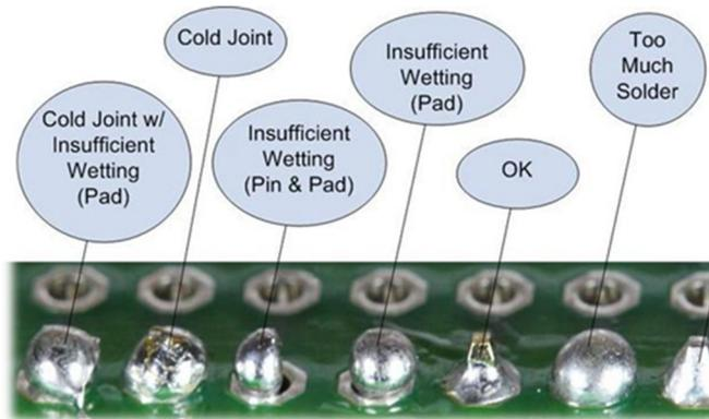
Figure 2 – Common soldering problems and their causes.
