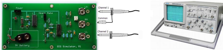
Figure 22 – ECG Simulator output measurement with an oscilloscope. The common contact from channel 2 does not need to be used, since this cable is connected to channel 1’s probe.
