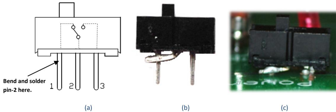
Figure 18 –Slide switch internal connection (s), pin 1 and 2 soldered (b) and picture of the ON/OFF power position.
