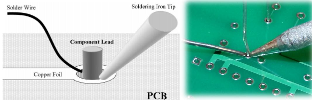
Figure 3 – Correct heating of component lead and hole, touching solder to joint and not the soldering iron.
