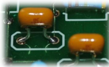
Figure 11 – Ceramic capacitors soldered to the PCB; these kind of capacitors do not have polarization restrictions.
