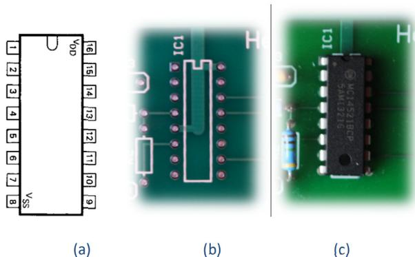
Figure 15 – Integrated Circuit outline drawing (a), silk screen (b) and chip placement (c).
