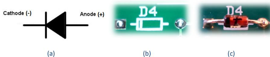
Figure 12 – Diode schematic symbol (a), location on the PCB before (b) and after (c) installation.
