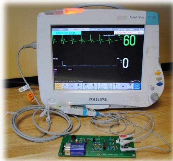
Figure 25 – EWH’s Kit connected to a real electrocardiogram machine. The number 60 corresponds to the simulated heart rate.
