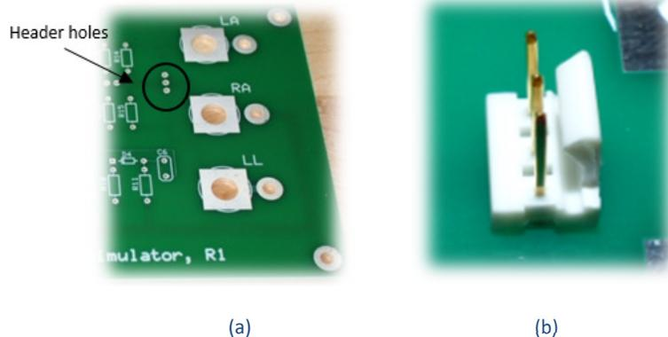
Figure 17 – Header contact position (a) and picture (b). The header contact allows the ECG signals to be connected to the case (not included in the kit).
