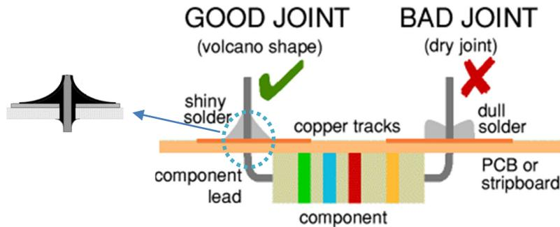
Figure 4 – Cross section view of the PCB in the soldering point.
