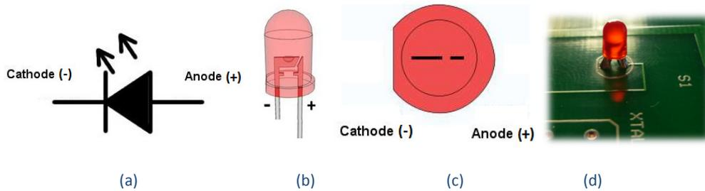
Figure 13 – Light emission diode (LED) schematic symbol (a), appearance (b), PCB representation (c) and picture (d).
