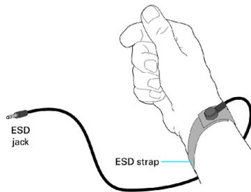
Figure 1 – Electrostatic discharge protection strap.
