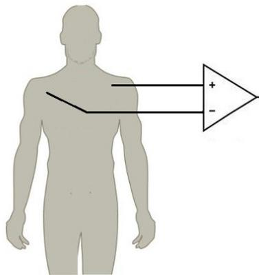
Figure 28 – The ECG measurement circuit uses a differential amplifier to subtract the voltages between the right and left arm (BotMultichill via Wikimedia Commons).
