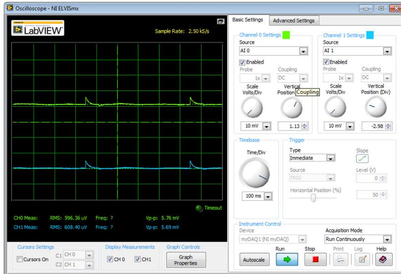
Figure 24 – NI ELVISmx Oscilloscope display and control panel.
