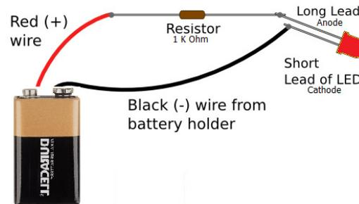
Figure 14 – Basic LED test procedure, the resistor value can change as long as it is higher than 1 k $\Omega$  (to avoid burning the diode).
