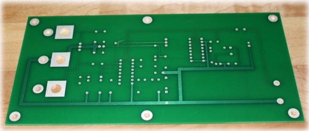
Figure 7 - Bottom layer of the bare PCB; the thicker via corresponds to the floating common, which is connected to the negative contact of the battery.
