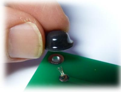
Figure 20 - Rubber feet to be placed underneath the corner holes.
