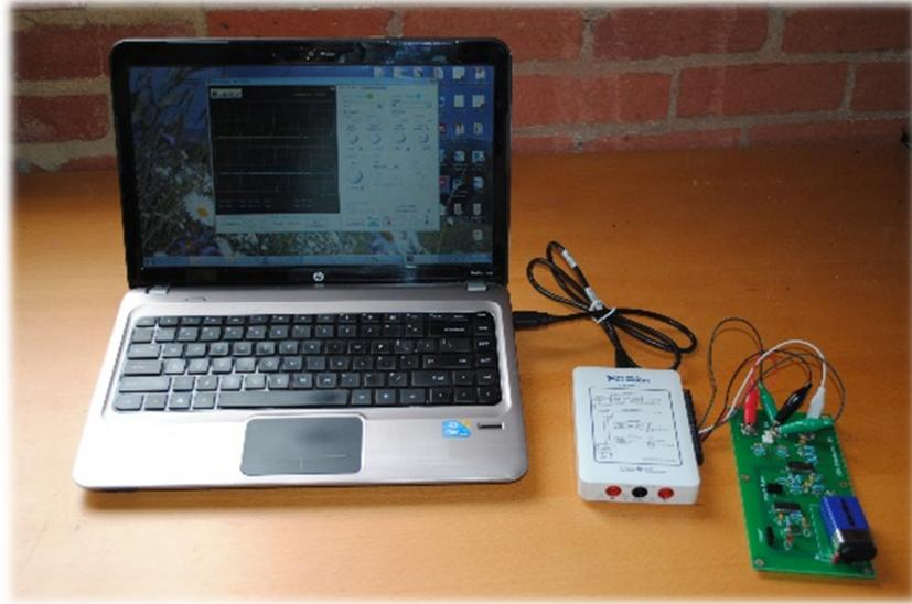
Figure 23 – ECG Simulator Kit measurement with National Instrument MyDAQ board.
