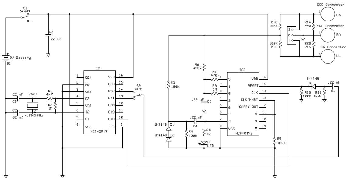
Figure 9 – ECG Simulator electronic schematic diagram. The 9 V battery is NOT included in the Kit!
