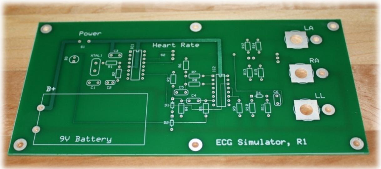
Figure 6 - Top of the bare printed circuit board with silkscreen marks to assist in placement of the electronic parts.
