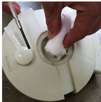
Figure 3.20: Placing the rolled gauze filter in place of the original filter.
