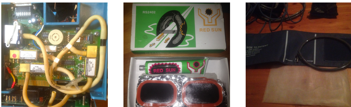
Figure 3.1: Aged tubing was one of the most common and simple fixes we encountered. Left: A Vital Signs Monitor, illustrating the amounts of tubing often found in medical equipment. Center: Aged rubber can simply be fixed using normal vulcanizing rubber bicycle patches. Right: A typical blood pressure cuff that can be repaired using bicycle patches as the bag is made of plastic. 5.6
