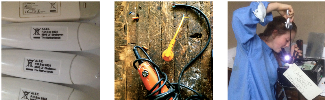
Figure 3.3: Left: Four broken thermometers we were given by the medical ward, which all worked after changing the batteries. Center: Cast cutter that needed a different plug. Right: Tubing often stretches and cracks over time, increasing the likelihood of leaks. Here, Ashley is repairing an automatic blood pressure monitor by replacing the old tubes with newer tubing cannibalized from an old blood pressure cuff.
