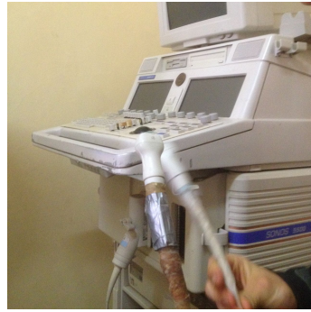
Figure 5.2: A problem commonly seen in ultrasound machines is damage from stress and strain at the junction of the cable and transducer cord.
