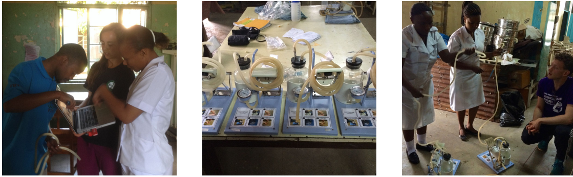
Figure 3.22: Left: Manual suction pumps at Mawenzi hospital that had been repaired. KJ discusses the details of the quick start manual with a nurse from the medical ward. Centre: Correct use of the manual suction pump requires some special techniques as described in the quick start guide. Right: The quick start guides were supplemented by hands-on training with nurses from each department at Mawenzi hospital.
