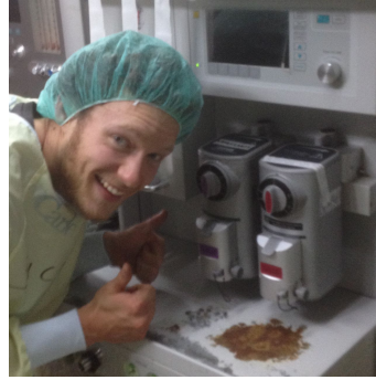
Figure 3.14: The isofluorane vaporizer was put back into the anaesthesia machine and is now in use in the surgical department.
