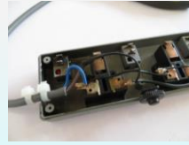
(3) Use zip ties to hold cable in place
