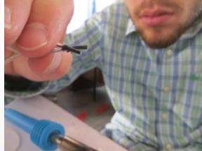
(2) Combine the two for one working temperature probe; use heat shrink to protect wires from shorting and provide strength
