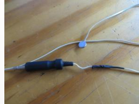
(2) Combine the two for one working temperature probe; use heat shrink to protect wires from shorting and provide strength
