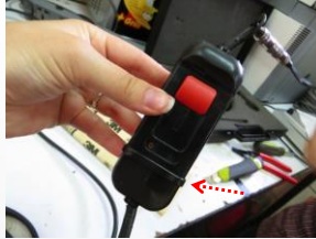
(2) Solder wire; secure with heat shrink; secure remote with zip tie
