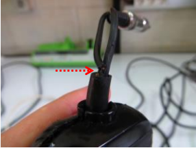
(1) One of the wires completely disconnected
