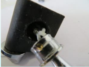
(2) Live inside of connector broken
