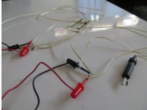
(1) Two broken temp. probes for infant warmer; 1 without sensor & 1 with broken plug
