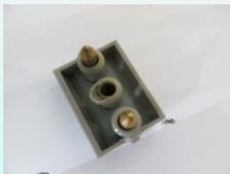
(1) Switch broken; used epoxy to hold pin in place
