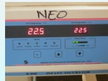
(4) Test unit; all alarms work; holds set temp.
