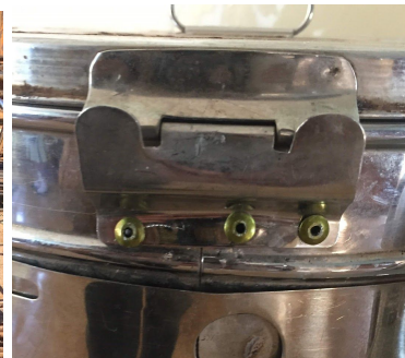
Repaired Autoclave Hinge
