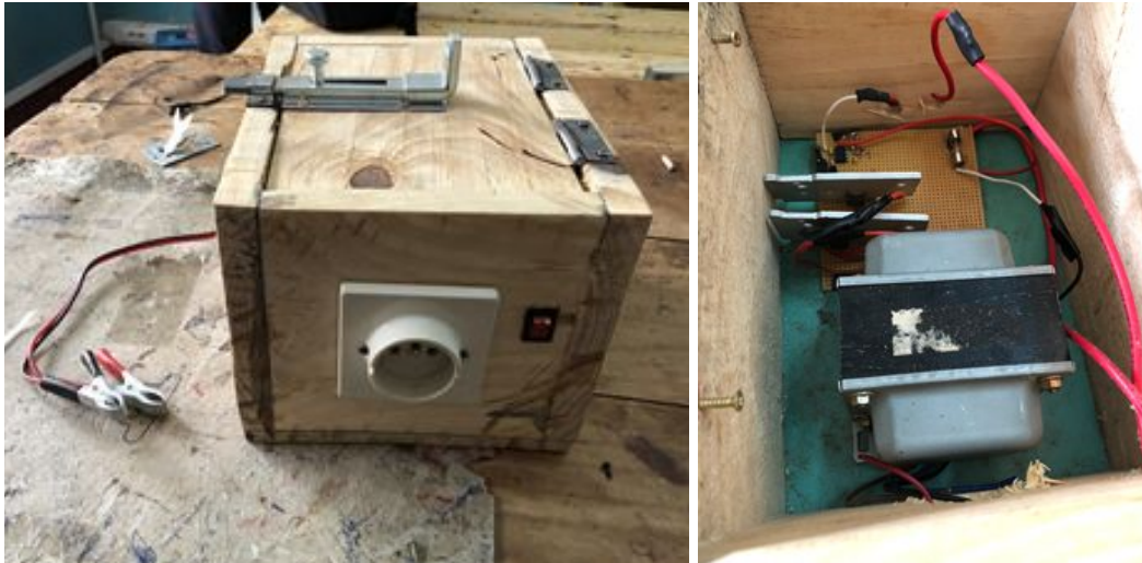
Exterior and Interior Views of the Inverter
