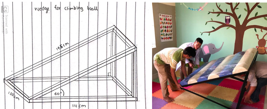
Climbing wall design; climbing wall installed with help of hospital staff
