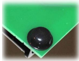
Figure 12: Rubber feet placed underneath corners of PCB.
