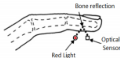
Figure 1 – Heart Rate measurement principle through the finger tip.
