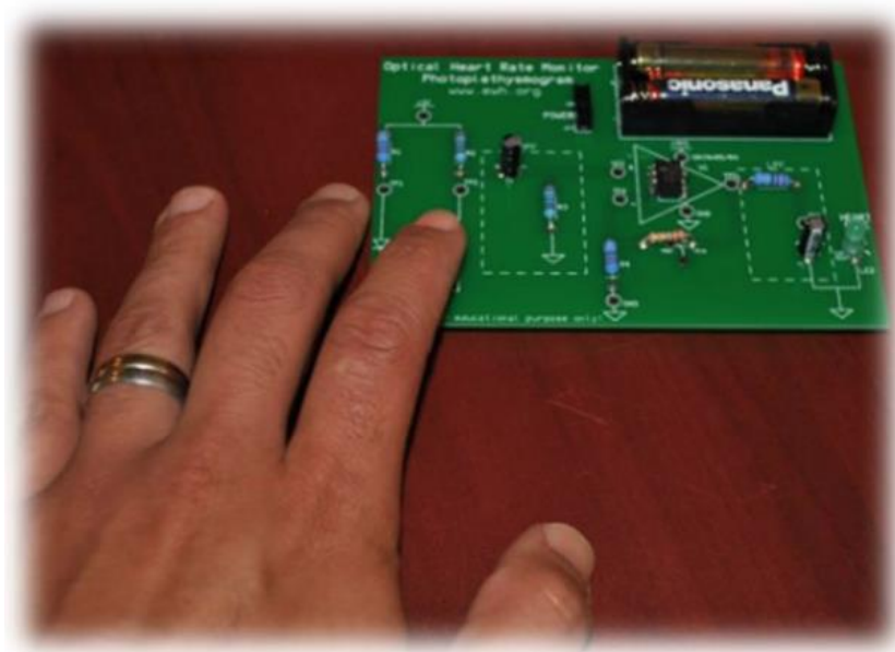
Figure 15: OHRM fingertip measurement. Make sure that all other fingers and elbows lay on the table.
