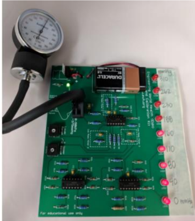
Figure 17: Gauge connected to the pressure sensor ‘positive pressure’ inlet.
