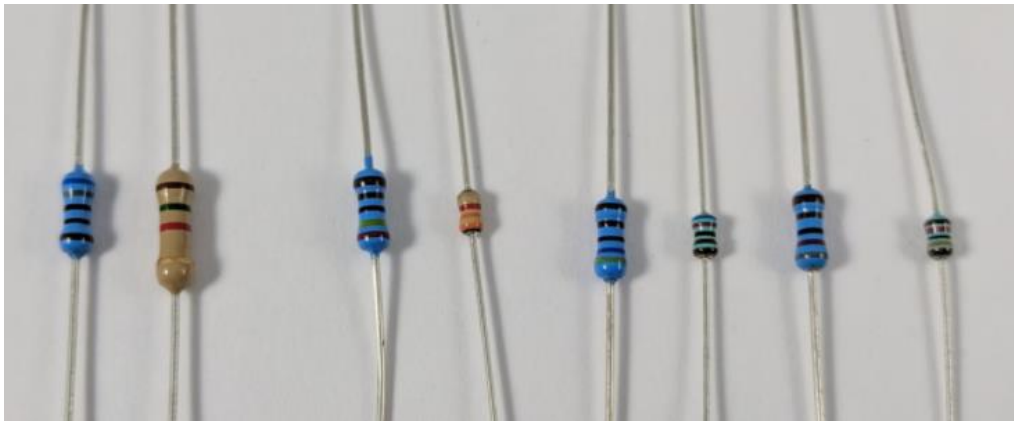
Figure 7: Comparator resistors in increasing order of resistance: 680 \Omega , 1.5 k \Omega , 2.4 k \Omega , 3.3 k \Omega , 4.7 k \Omega , 6.2 k \Omega , 8.2 k \Omega , and 13 k \Omega . Clever observers might note that there are only eight resistors, but nine LED indicators. This is because the ninth comparator uses a 10 k \Omega resistor, which was already soldered on at R31.
