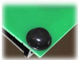
Figure 14: Rubber feet placed underneath corners of PCB.
