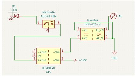
Figure 5. Compressed schematics of the surgical lamp without resistors and capacitors. Diagram shows the AC to DC inverter connected to the ATS where the output is connected to the manual switch of the surgical lamp [14].
