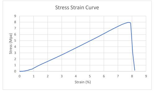
Figure 8: Stress Strain Curve for Track Adapter
