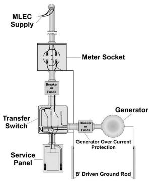
Figure 6: Schematic diagram of a generator transfer switch. Demonstrates how an electrician would normally install a transfer switch [15]
