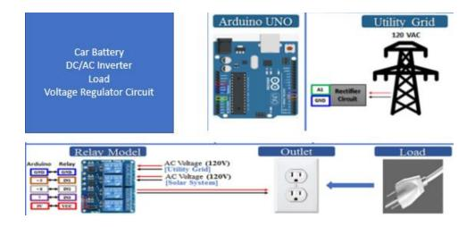
Figure 7: Block Diagram of Automatic Power switching with Arduino Uno [17]
