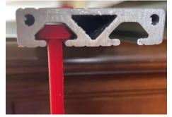
Figure 3: 3D-Printed Adapter in 80/20 Track
