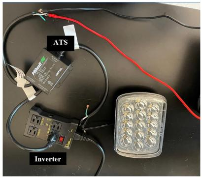
Figure 10. Built circuit containing the ATS
