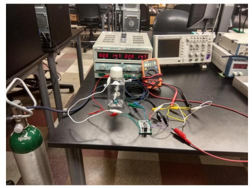
*Figure 4*. Air Containment Device Testing to see if current-oxygen concentration relationship can be reproduced.
