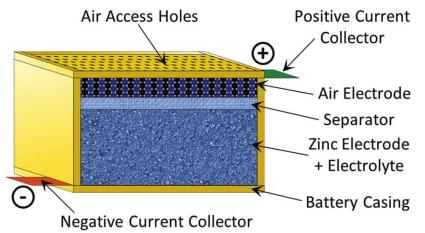
*Figure 1.* Zinc-Air Battery Diagram. Taken from: Fu, J., Cano, Z. P., Park, M. G., Yu, A., Fowler, M., & Chen, Z. (2016). Electrically Rechargeable Zinc-Air Batteries: Progress, Challenges, and Perspectives. *Advanced Materials*, *29*(7), 1604685. doi:10.1002/adma.201604685
