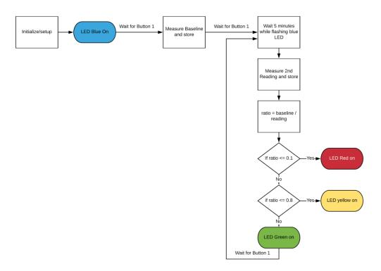
Figure 3. Code Block Diagram for Microcontroller.
