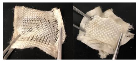
**Figure 2.** Preliminary filter design used in Proof of Performance tests. Left image shows one layer of knitted polymer mesh. The layers can be stacked to create a multilayered woven filter (right image). The individual polymer fibers are pulled and then coated with silver nanoparticles. The weaving of the strands for each layer controls the pore size for an individual mesh layers.
