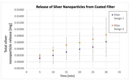
Figure 3. Release of silver nanoparticles from the prototype (single layer) woven mesh filters.
