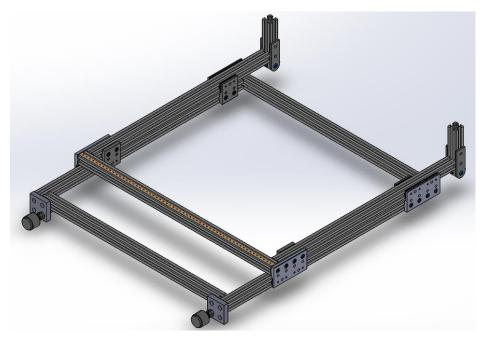
Figure D.2 - Digital model of leg subassembly Appendix G – Parts List
