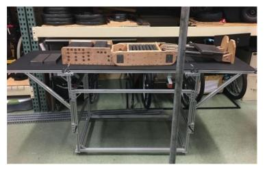
*Figure 2: Testing the table with an ISO-standard dummy according to IEC standards.*
