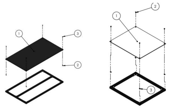
*Figure C.1 - (Left) Central tabletop subassembly. (Right) Folding tabletop subassembly.*
