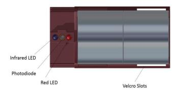
Figure 2. Bottom View of the Prototype
