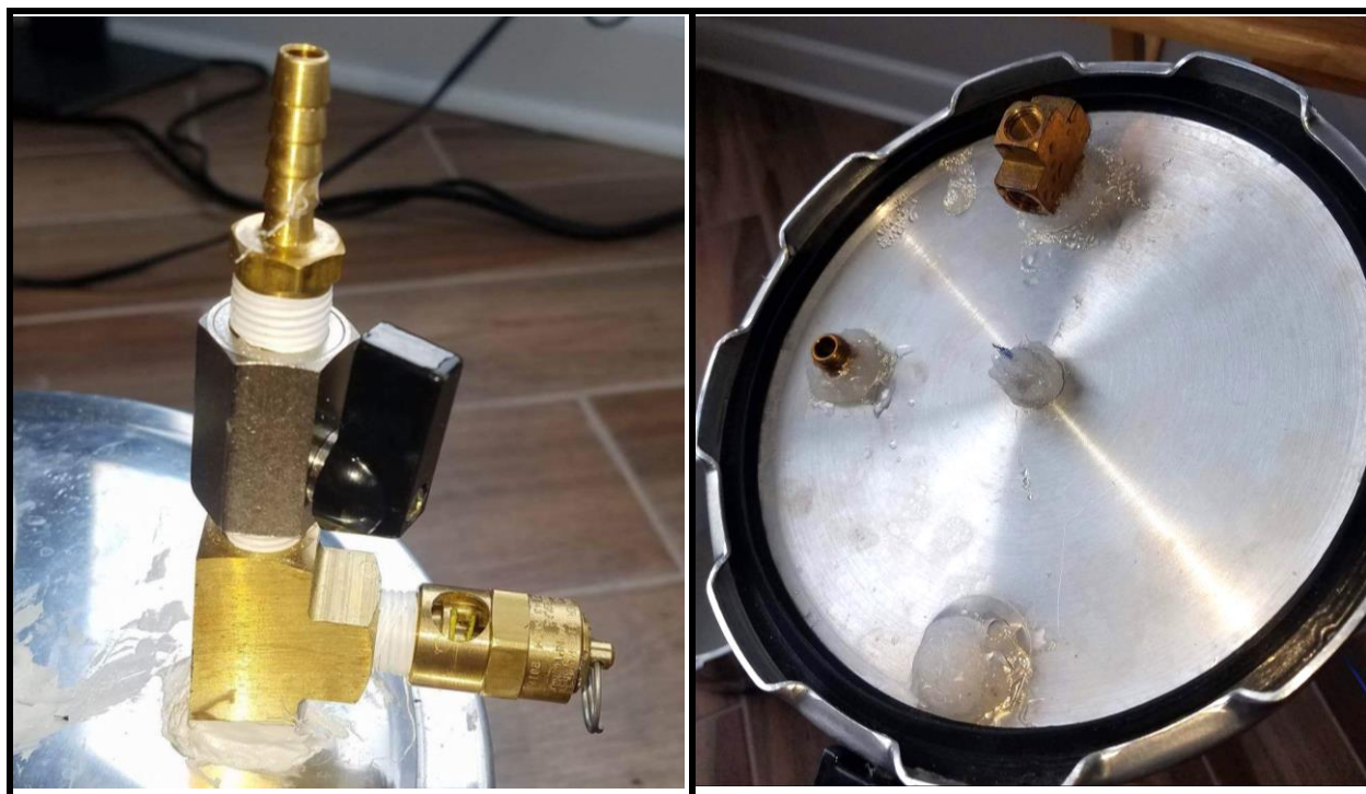
Figure 1. The autoclave, built from a modified pressure cooker (A) Modified pressure cooker (B) Pressure gauge attached to the lid of the autoclave (C) Safety valve, ball valve, and vacuum fitting attached to the lid of the autoclave (D) Silicone sealants used on the underside of the lid to prevent air leaks
