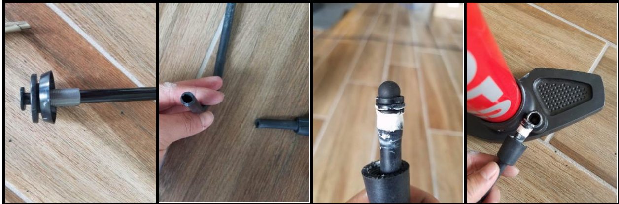
Figure 2. The vacuum pump, built from a modified bicycle pump (A) Hose is removed (B) Base is removed (C) Top is unscrewed (D) Plastic and rubber assembly is removed (E) Rubber piece is reversed and reattached (F) hose is cut (G) ball valve is reversed (H) Ball valve is reinserted.
