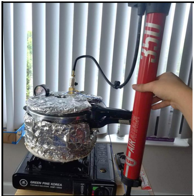
Figure 3. Completed autoclave with insulation and vacuum pump.
