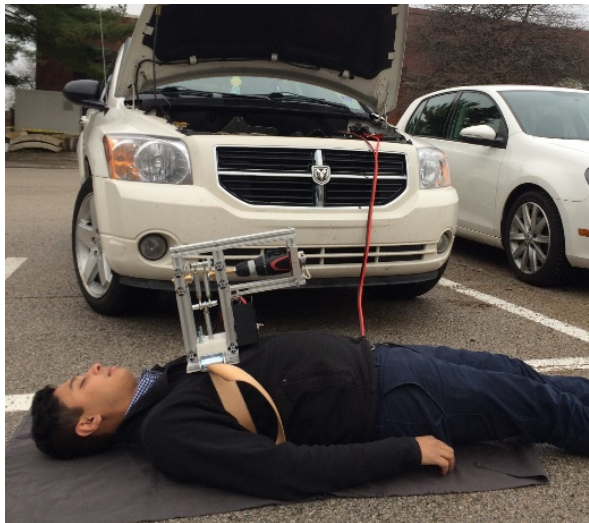
Figure A.4.2: Shows how the device can utilize a car battery for power
