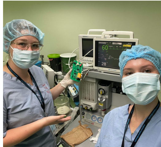
Testing a patient monitor using an ECG simulator
