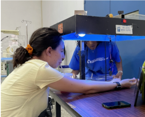
Replacing blue-colored white bulbs in a bili light with blue LEDs to make it more effective
